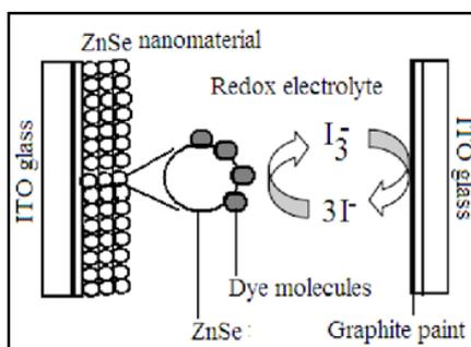
**Figure 1: Schematic Overview of a Dye Sensitized Solar Cell**
