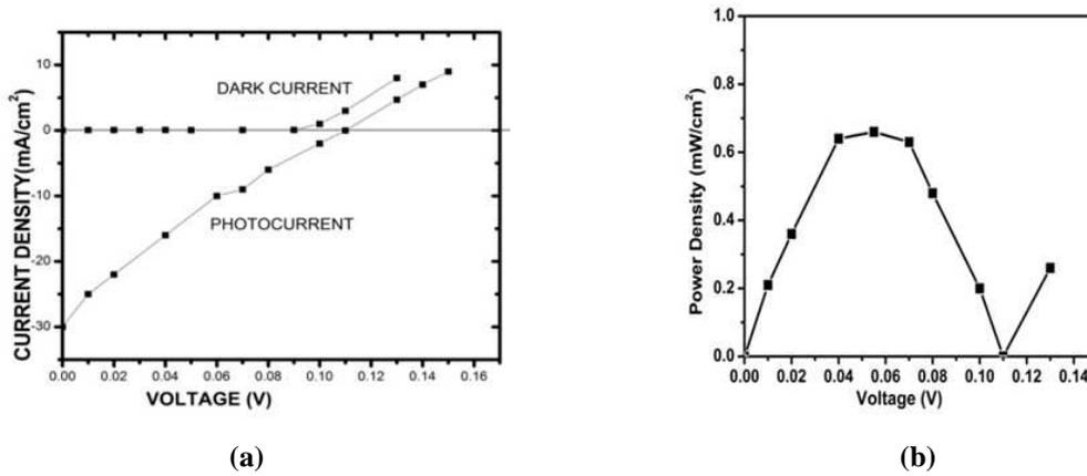
Figure 7: (a) Current Density (J) Vs Applied Bias (V) Characteristics and (b) Power Density (P) Vs. Voltage (V) Plot Fill Factor and Efficiency Can Calculated from the Relation Given Below
