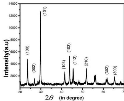
**Figure.3: XRD Pattern of as Synthesized Znse Nanoparticles**
