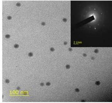
**Figure 2: The TEM Image and Sad Pattern of as Prepared Nanoparticles**
